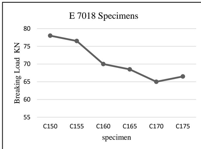
Hence, from the graph and the result table we can conclude that the specimen with current of 150 Amp i.e. C150 has the highest load bearing capacity
