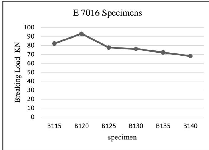
Hence, from the graph and the result table we can conclude that the specimen with current of 120 Amp i.e. B120 has the highest load bearing capacity
