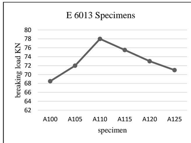
Hence, from the graph and the result table we can conclude that the specimen with current of 110 Amp i.e. A110 has the highest load bearing capacity
